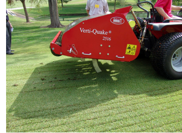
Verti-Quake Blades "Fracturing" the Soil Profile
